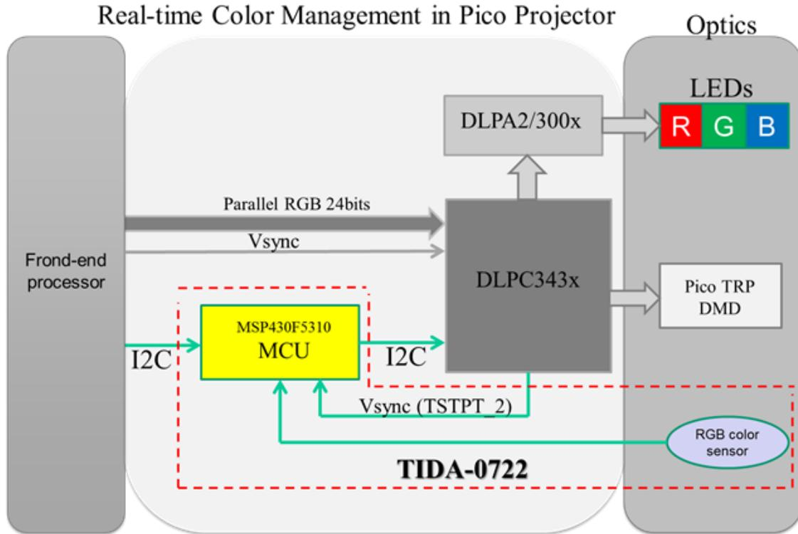
MSP430F5310 MCU runs the real-time color management algorithm as the critical role that interacts with DLPC3439 for LED current correction and updating color-related registers based on color sensor feedback in frame-basis per the given desired color targets. Please note that performance will vary across EVMs due to variations in manufacturing. The performance data is not guaranteed.
