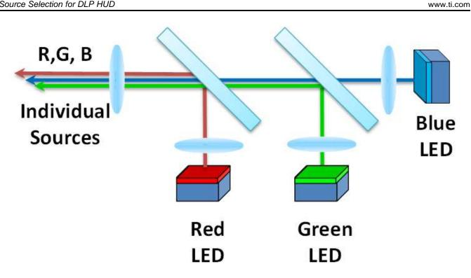
Figure 6. Typical LED Sequential Illumination
