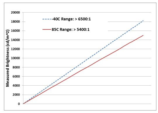
Figure 8. Measured Light Output for DLP HUD
