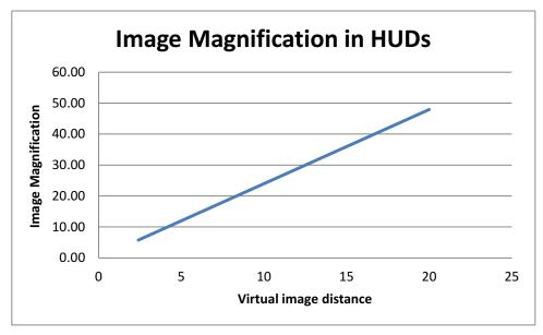
Figure 3. Image Magnification vs Image Distance
