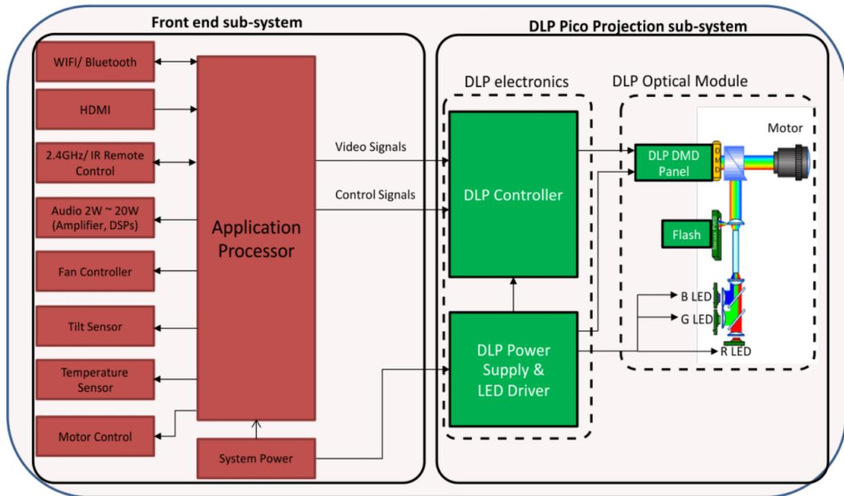
*Figure 4. Screenless Display System Diagram*
