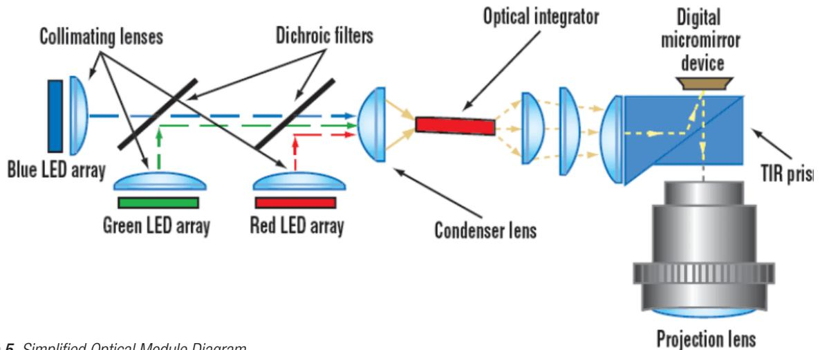
**Figure 5.** Simplified Optical Module Diagram
