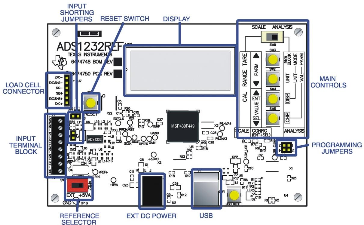
Figure 6. ADS1232REF Weigh Scale Reference Design Layout
