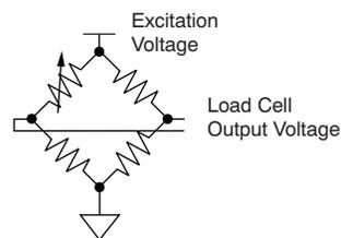
**Figure 1. Wheatstone Bridge Resistive Load Cell**
