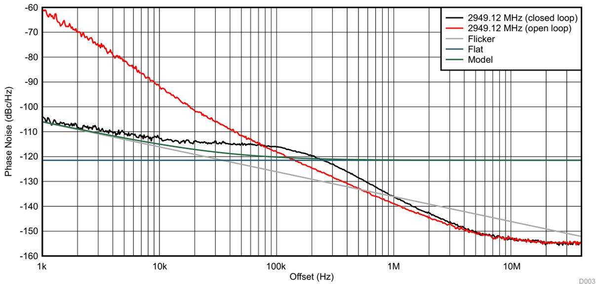
Figure 5. Sampling Clock of 2949.12 MHz With 58 fs Jitter
