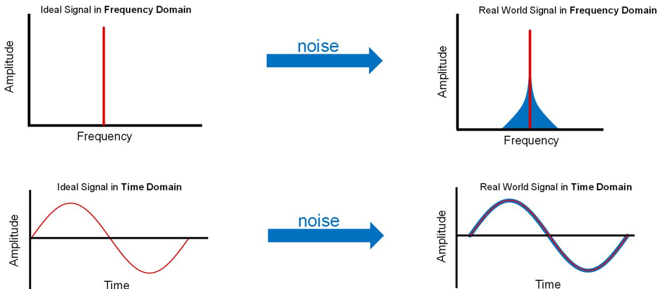
Figure 3. Phase Noise in the Frequency and Time Domain
