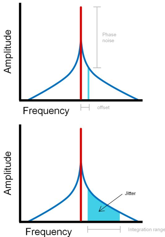
Figure 4. Phase Noise and Jitter Definitions
