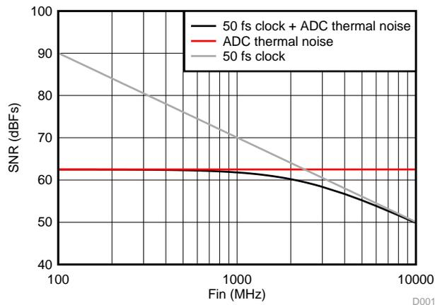
**Figure 1. ADC and Clock Jitter Contribution to SNR**
