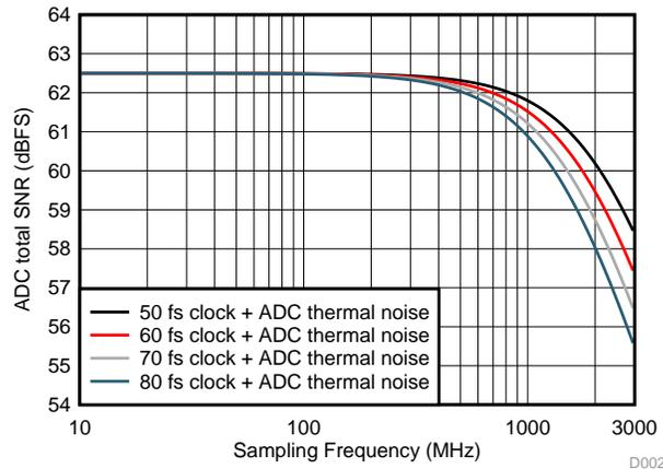
Figure 2. Impact of Different Clock Jitter to Total SNR
