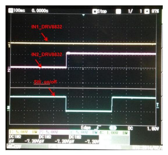
In the above figure, the signals illustrate the situation when the flip up display is commanded to OPEN. The user switch (SW\_on/off) is pressed, IN1 is low, IN2 is high, and the flip up display opens. The oscilloscope is set to trigger off of the user switch (SW\_on/off).
