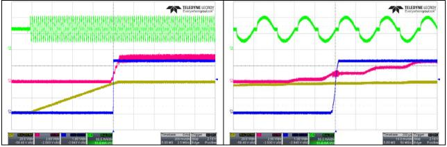
Channel 1 VIN<sub>DC</sub> Channel 2 Enable Channel 3 VOUT Channel 4 IIN<sub>AC</sub>
