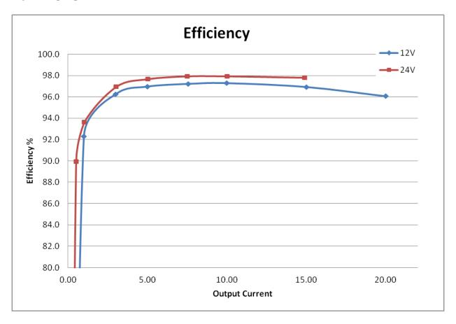
Efficiency can be dependent on the type of inductor used. The following plots indicate efficiency change with inductor type:
