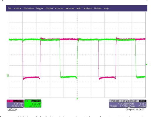
12V System, 10A Load. Individual channel switch nodes show interleaved operation
