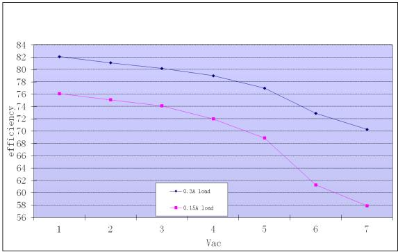
2.2.2 efficiency curve at 5% and 10% of full load
