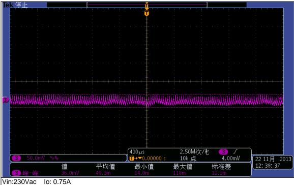
Ch3: output ripple voltage, 50mV/div
