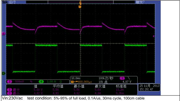
Ch3: output voltage Ch4: output current
