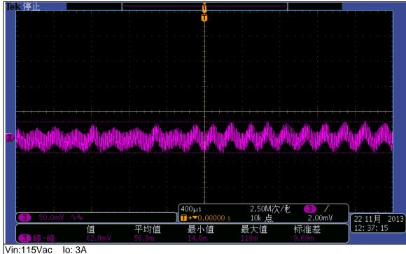
Ch3: output ripple voltage, 50mV/div
