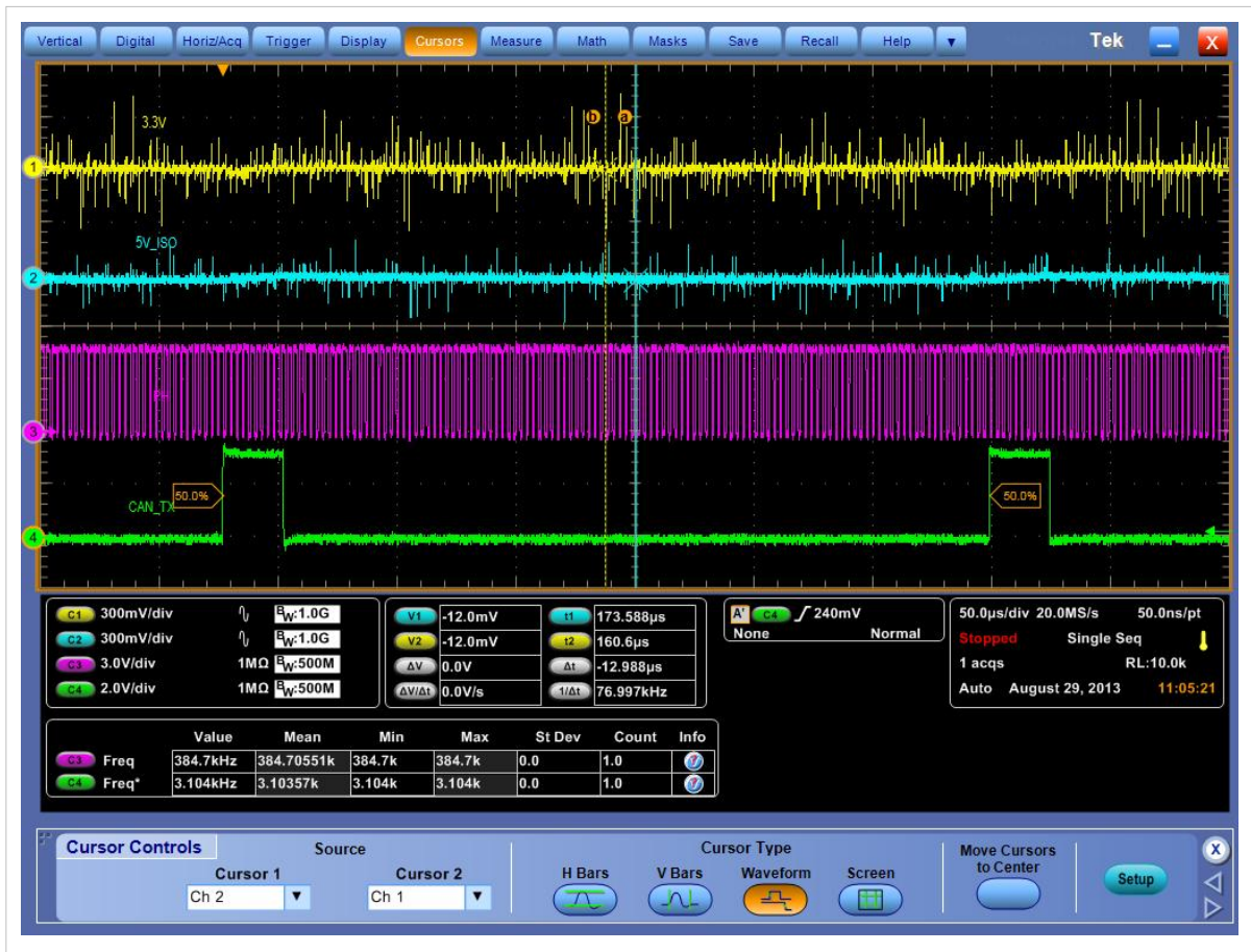
Figure 8: Output Ripple and PH node with EN enabled, CAN (37 kbps, 11 bits low, 1 bit high)
