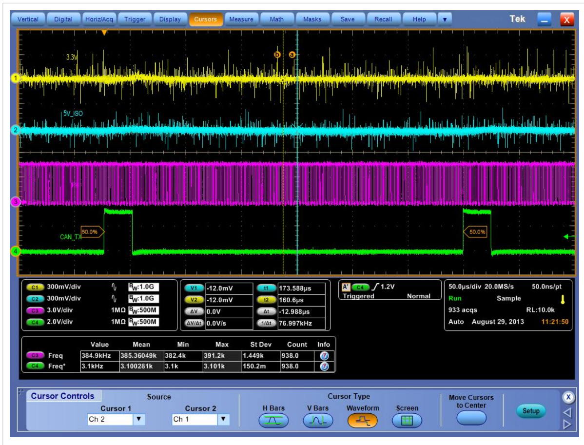
Figure 12: Output Ripple and PH node with EN enabled, Profibus (12 Mbps), CAN (37 kbps, 11 bits low, 1 bit high)
