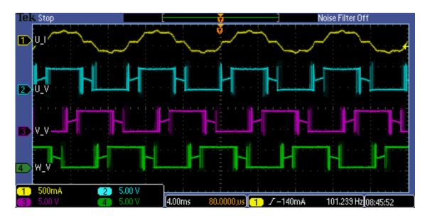
Section 2: 3-Phase Sensorless Commutation Scheme\_2
