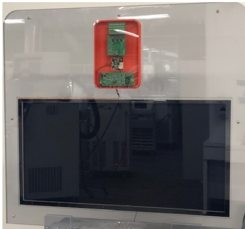
图 16. Test Setup of SPD-SmartGlass and TIDA-020013 mounted together
