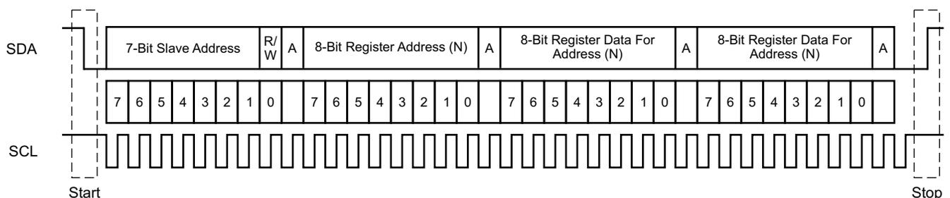
Figure 16. Typical I<sup>2</sup>C Sequence
