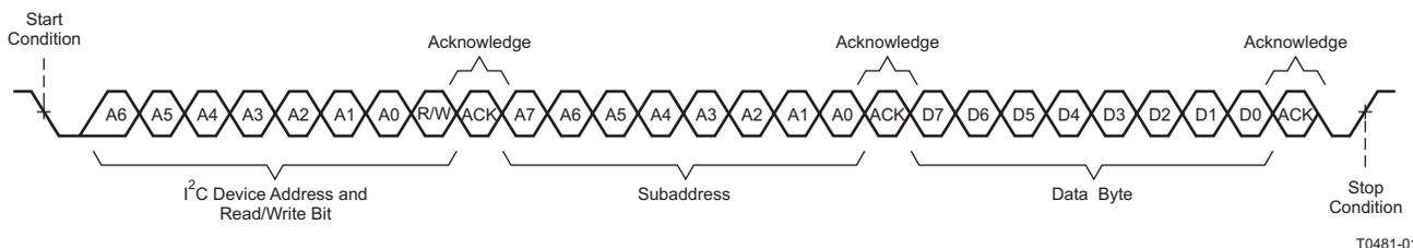
Figure 17. Single-Byte Write Transfer
