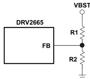
The boost output voltage is given by [Equation 1](#), where  $V_{FB} = 1.32 \text{ V}$ .
