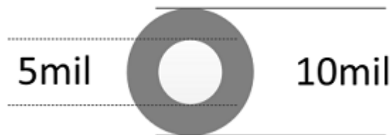
Figure 88. Under Ball Recommended Via Size
