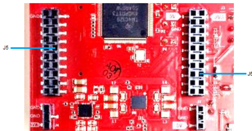
Figure 5. 20-Pin BoosterPack Connectors
