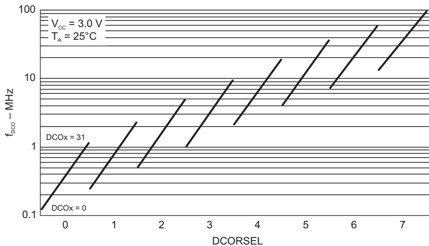
Figure 5-15. Typical DCO Frequency
