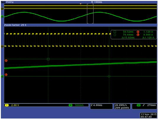
Figure 10. Test waveform (Motor2 1/128 I\_level\_2)
