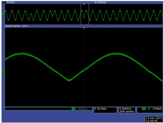
Figure 12. Current waveform when change DIR
