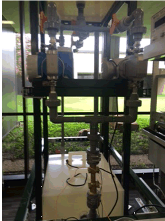
Figure 17. Flow Test Setup
