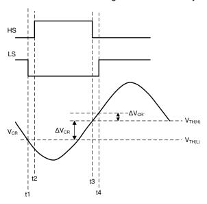
Figure 4. HHC Gate Control Principle
