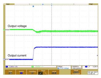
Figure 8. HHC Transient Response
