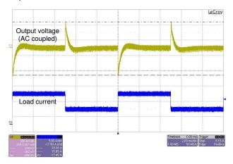
Figure 1. Transient Response Example
