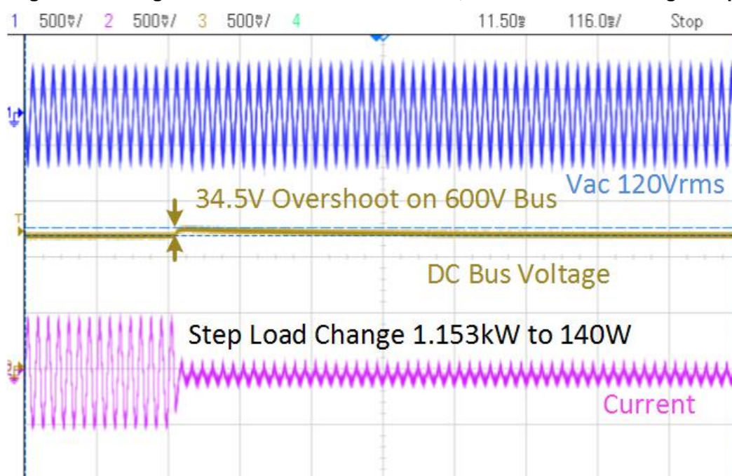
Figure 65. Voltage Overshoot With 1-kW Transient, With Non-Linear Voltage Loop
