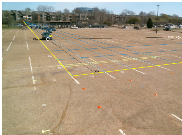
Figure 35. Translating Pixels to Real World Coordinates
