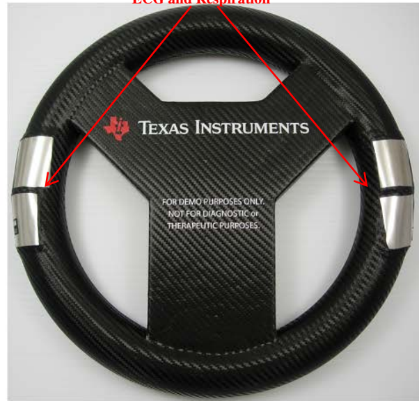
Electrodes on Biometric Steering Wheel used for ECG and Respiration
