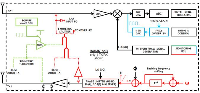
Figure 3. On-Chip TX-RX Test Signal Loopback Architecture: TX Monitoring, RX Monitoring, RX Baseband Monitoring
