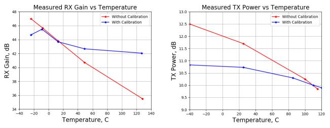
Figure 2. RX Gain and TX Power With and Without Calibration
